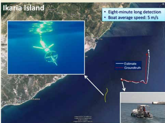
Figure - Example of experimental result achieved at sea during PERSEUS final demo (Eastern Campaign, Sept. 2014). During one of its missions (glider track in yellow line) the glider detected and localized a small boat crossing the area (boat trajectory: true in red, estimated in white).
