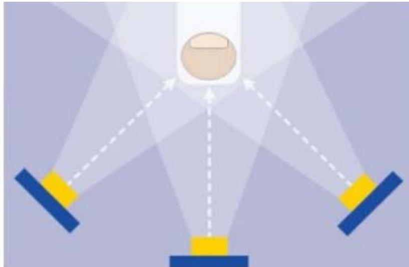
Figure 53: Schematic View Touchless Fingerprint Scanner<sup>50</sup>
