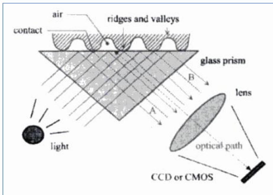
Figure 51: Principle of optical sensor<sup>46</sup>
