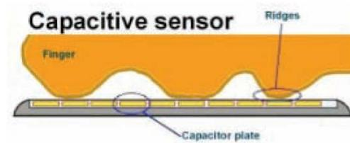
Figure 50: Principle of capacitive sensor<sup>45</sup>
