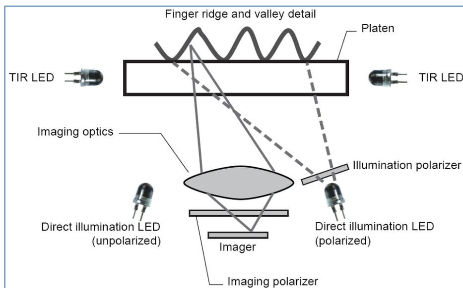
Figure 52: Schematic principle of multispectral sensors<sup>49</sup>
