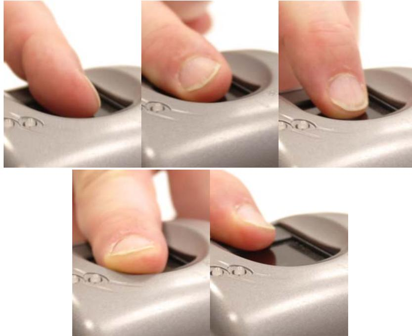
*Figure 4: Wrong positioning of the finger on a scanning device
