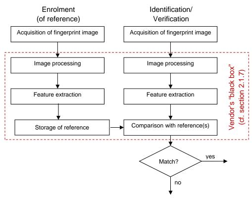
Figure 2: Fingerprint recognition process
