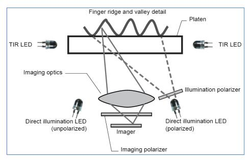
Figure 52: Schematic principle of multispectral sensors<sup>49</sup>
