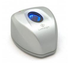
Figure 40: Multispectral sensor from Lumidigm<sup>27</sup>
