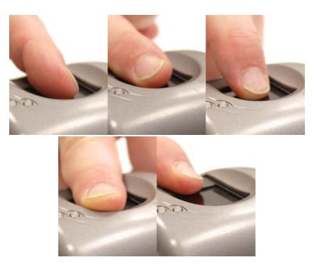
Figure 4: Wrong positioning of the finger on a scanning device (too far turned to left side; too far to right side; too steep; too much advanced; too less advanced)
