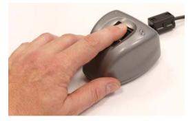
Figure 3: Acquisition of a fingerprint from an index finger by a commercial scanning device
