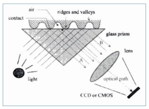
Figure 51: Principle of optical sensor<sup>46</sup>
