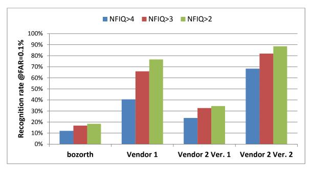
Figure 25: Recognition rates vs NFIQ of the tested algorithms
