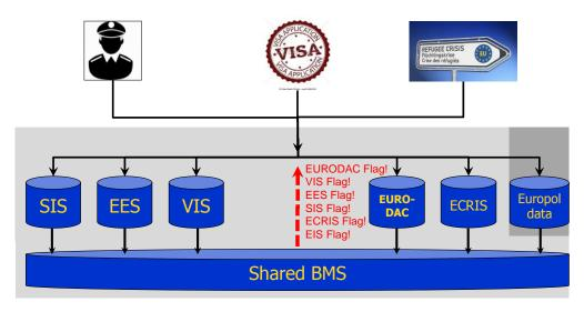
Figure 5: Shared biometric matching service (BMS) with 'hit flags'
