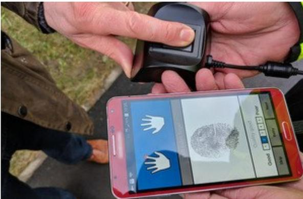
An app on an officer's phone, combined with a handheld scanner, will mean police will be able to check fingerprints against both criminal and immigration records by connecting to the two live databases (IDENT1 and IABS) via the new Biometric Services Gateway.
